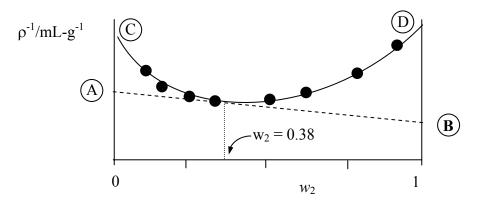
The intercept A is:  $\tilde{v}_1$  (at  $w_2 = 0.38$ ). It is appreciably different from the inverse of the pure solvent density, located at point C.
