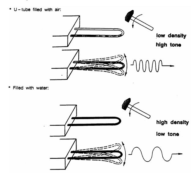
How good is the DMA 58? Damn good! From its manual: "...an accuracy of  $\pm 0.00002$  g/cm<sup>3</sup> within a measuring range from 0.5 to 1.5 g/cm<sup>3</sup>..." under typical calibration conditions.
