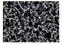
Cellulose acetate membrane (Type ST 68, 0.8 µm)
