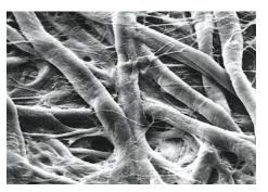
Cellulose filter papers exhibit particle retention levels down to 2.5  $\mu m.$
