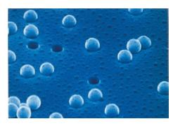
Microscope image of the surface area of Cyclopore™ PC polycarbonate membrane filters
