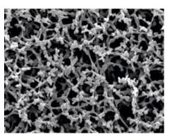
Cellulose acetate membrane (Type ST 68, 0.8  $\mu m)$
