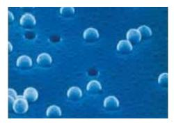
Electron micrograph of Cyclopore<sup>™</sup> membrane with latex beads on surface
